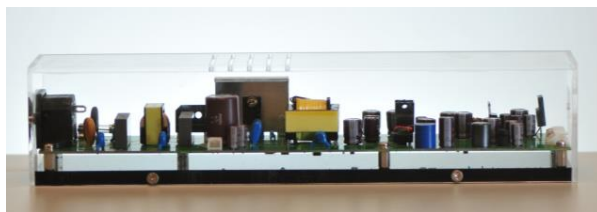
Figure 1.4 Flyback Auxiliary Power Module
