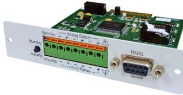
PEL-5000G series 9923 Current Waveform Generator & RS232 Interface
