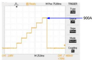
PEL-5006G-150-600 Turbo mode ON OCP Istep 30A, Istop 900.0A real test waveform
