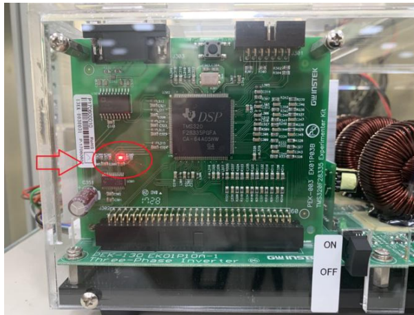
Figure 2.19 DSP normal status with light on
