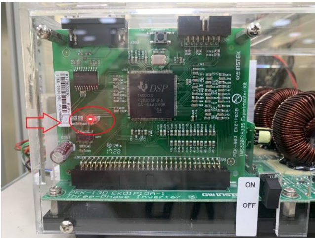
Figure 1.28 DSP normal status with light on
