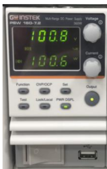
Figure 3.18 Power state of PSW and APS-300 when no load
