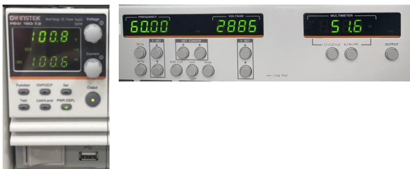
Figure 3.22 Power state of PSW and APS-300 when full load
