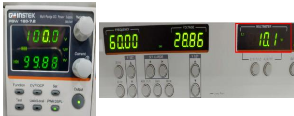
Figure 3.15 PSW and APS-300 power state under half load
