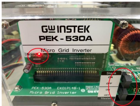
Figure 5.8 DSP normal status with light on
