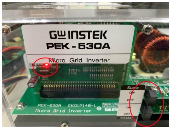
Figure 1.8 DSP normal status with light on
