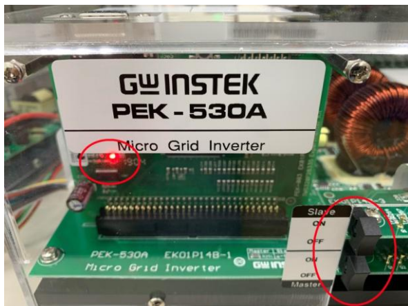
Figure 3.7 DSP normal status with light on
