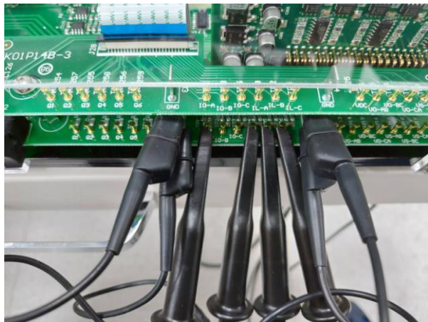
Figure 2.19 Oscilloscope test leads wiring
