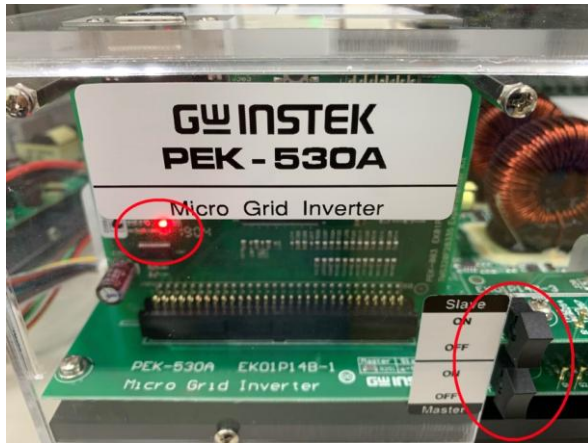
Figure 2.8 DSP normal status with light on
