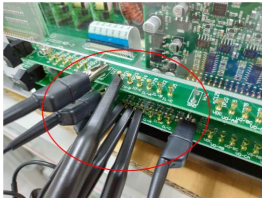
Figure 6.20 Oscilloscope test leads wiring
